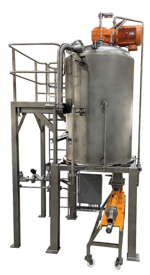
BCH has developed a 100% fruit cooking and extrusion system for the manufacture of healthy snack products. This is in response to the latest customer trends for natural, organic and clean ingredient labels.
