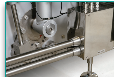
Cables run in sealed stainless conduit
