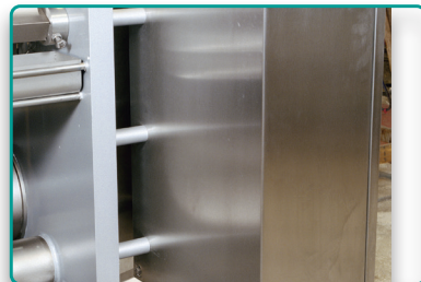
Holes eliminated where possible
