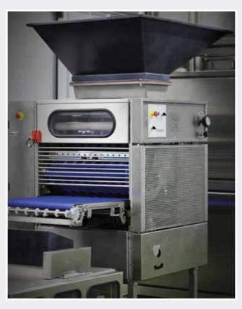
Approximate Machine Dimensions: 1200 mm (W) x 1100 mm (L) x 1600 mm (H), 900 mm standard table height, but can be adjusted to customer requirements
